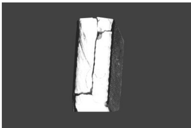
Figure 5 Photograph of sandwich composite failed under edgewise compressive loading.
